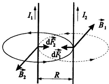
$$B_1 = \frac{\mu_0 \mu}{4\pi} \frac{2I_1}{R}, \quad dF_1 = I_2 B_1 dl.$$
